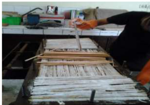
Figure 4. Layered in longitudinal and transversal with glue
